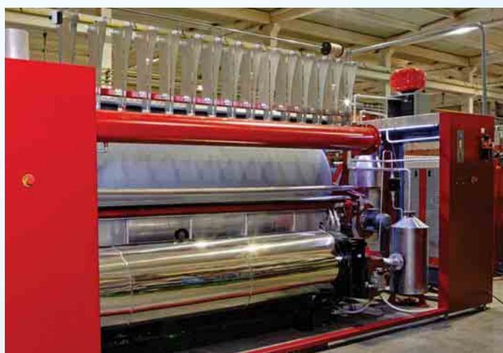
Gas heating system
